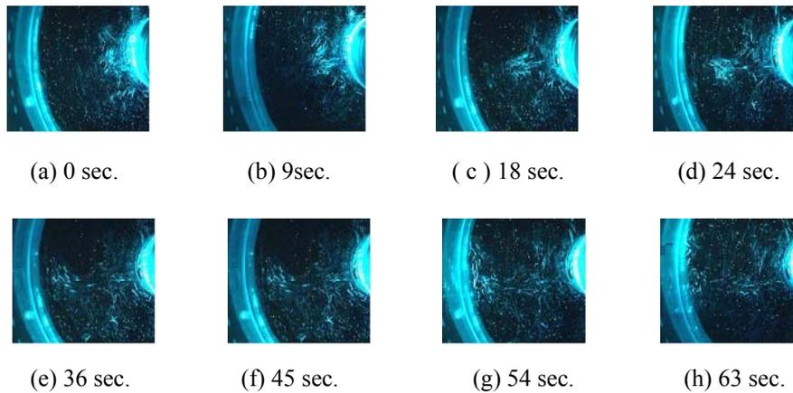
Fig. 4: Timewise variation of fiber motion in the rotating drum at 320 rpm.
