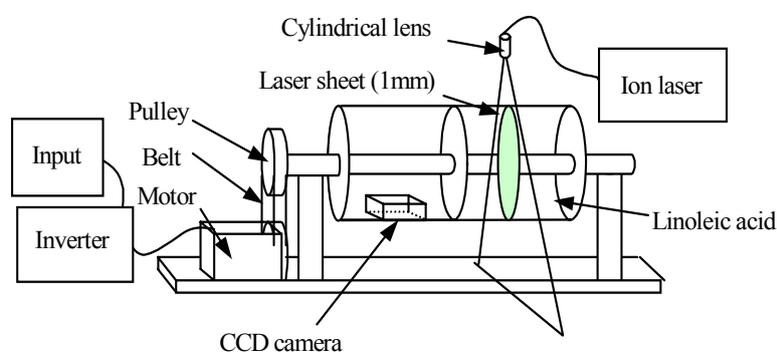
Fig. 1: A schematic of the experimental apparatus.
