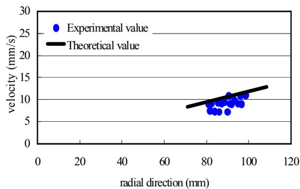
Fig. 8: Comparison of the measured particle velocity with the theoretical value.
