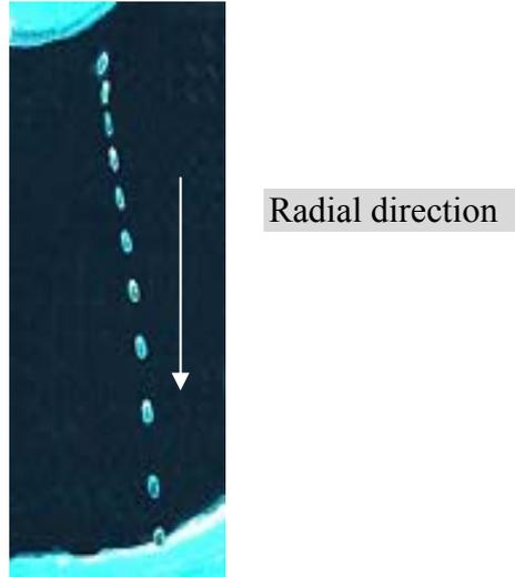
Fig. 7: Motion of circular disk in the rotating drum.
