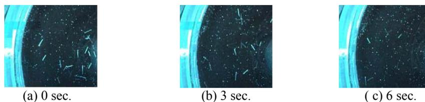
Fig. 3: Timewise variation of Fiber motion in the rotating drum at 640 rpm.
